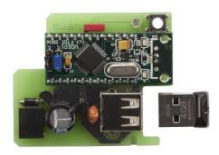
« plug-and-play » Installation in the communication slot for AMI transmitters (see limitations).
