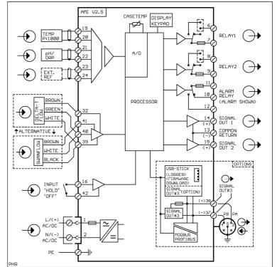
Transmitter temperature monitoring with programmable high/low alarm limits.
