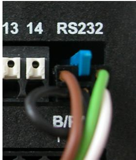
The AMU Interface RS232 PCB is used for Logger down load and Firmware up load. For detailed information see the corresponding manual “AMU RS232 Interface”.
