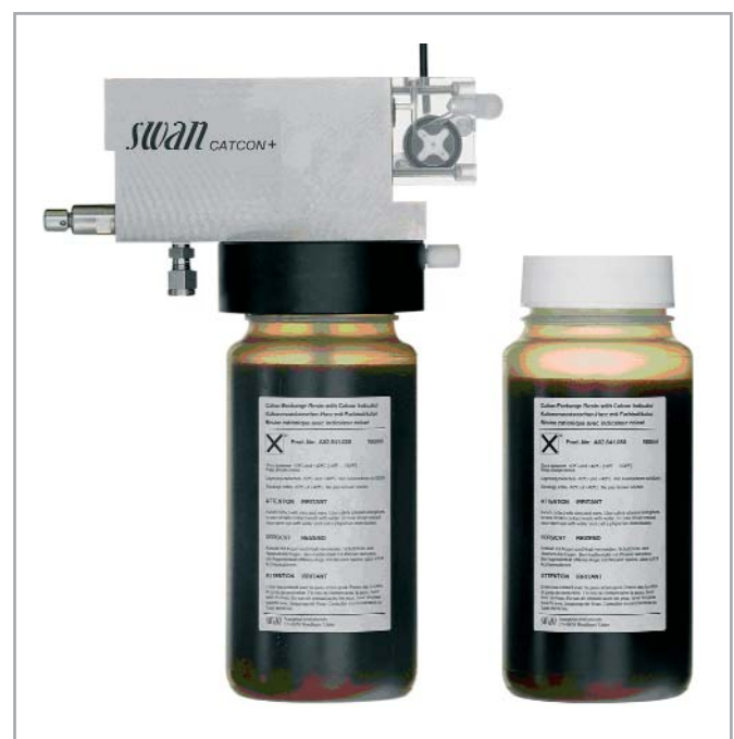
Figure 1: Catcon bottle used as an ion exchange column with a flow cell for two conductivity sensors with integrated needle valve and digital flow meter.
