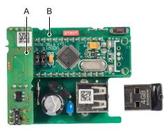
A Signal output 0/4–20 mA PCBB USB interface
